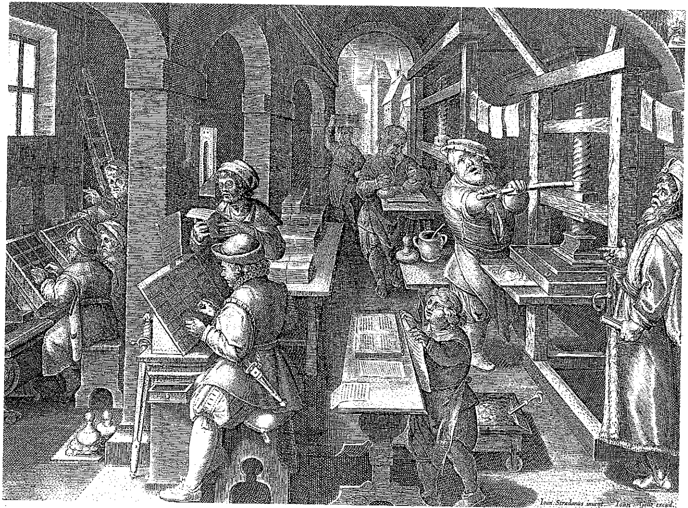
The Print Shop Sixteenth-century printing involved a division of labor. Two persons ( left ) at separate benches set the pieces of type. Another ( center, rear ) inks the chase (or locked plate containing the set type). Yet another ( right ) operates the press, which prints the sheets. The boy removes the printed pages and sets them to dry. Meanwhile, a man carries in fresh paper on his head. ( Giraudon/Art Resource, NY )
